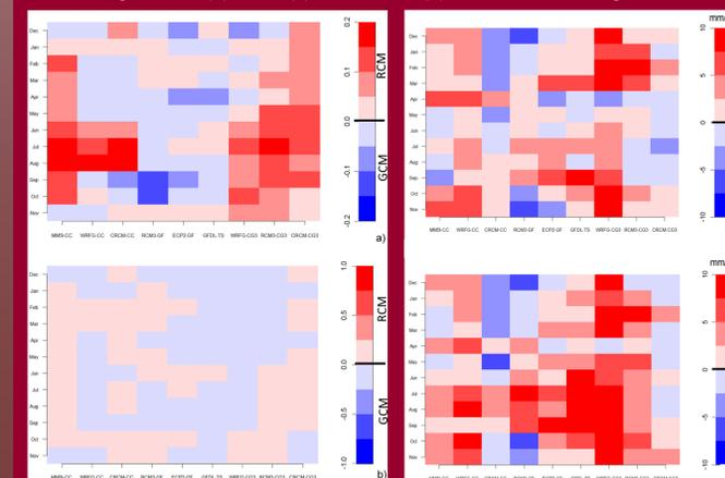
Figure 6: Value added for mean precipitation Perkins skill score (a), Willmott's index of agreement (b), MAE (c), and RMSE (d) for the east sub-region.
